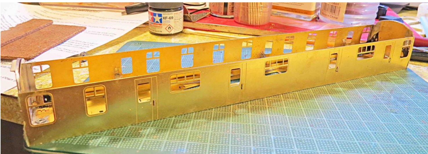
Successful trial fitting of the coach body on to the partially assembled floor.
